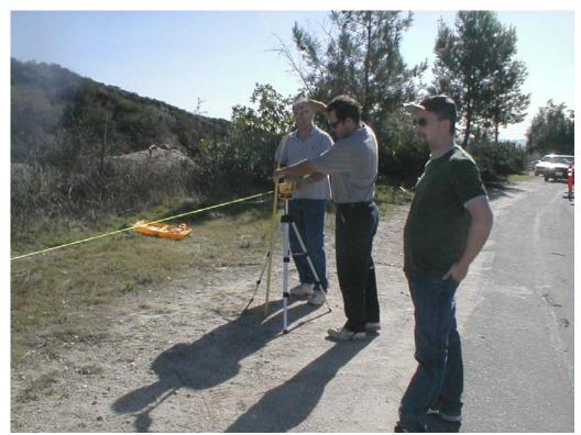
Measuring beam height at laser
